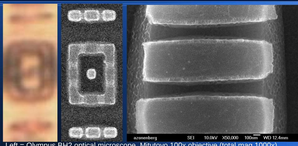
Left = Olympus BH2 optical microscope, Mitutoyo 100x objective (total mag 1000x) Center = JSM-6335 SEM, 2,500x Right = JSM-6335 SEM, 50,000x
