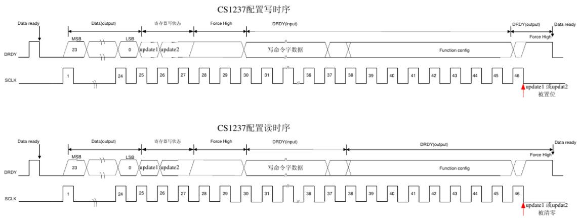
Figure 9: Function configuration timing diagram
